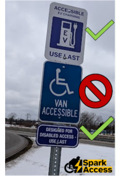
US Access Board Recommends Accessible Charging and “Use Last” Signage 13 that does not use the ISA to avoid conflict with other federal and state regulations. Ohio Turnpike
